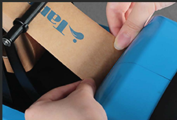
4. Insert the tape into the feed slot
